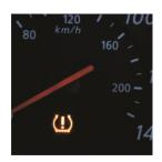
It's important to note that the in the cases of a nonfunctioning, not relearned or missing TPMS sensor, the TPMS MIL may not be evident. In other words, it can sometimes take a long while before a failed or missing TPMS sensor actually shows as a TPMS MIL [flashing light]. This makes
