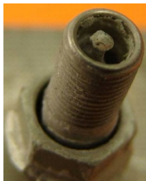
Heavily corroded sensor
