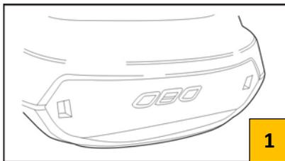
2. With your tool face up, insert the module with the longer 8-pin row of the OBDII connector at the bottom.
