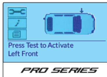
3. Continue with the Right Front, Right Rear, and Left Rear as the tool prompts you. The tool should indicate a successful read with "All Sensors OK".
