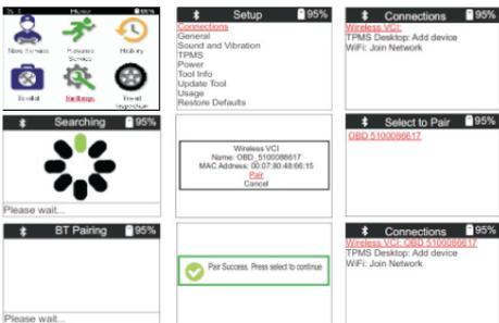
If using a secondary Wireless VCI please return to the connections page to remove the first VCI in order to pair a second VCI. **The Tech600PRO will only connect to ONE VCI at a time.**
