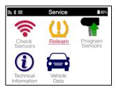
To find out which relearn type is available for a vehicle, just turn on the tool and select Relearn. Or refer to the current coverage list at <a href="https://www.bartecusa.com/tpms-tool-coverage-charts">https://www.bartecusa.com/tpms-tool-coverage-charts</a>.
