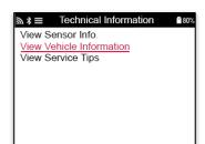
**View Vehicle Information**This option provides information about the Relearn method, the OBD port location and if there are programmable Sensors for the preselected MMY available.
