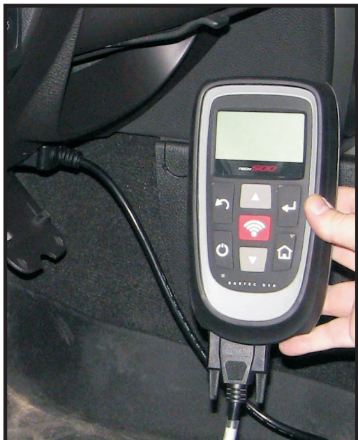
Tech500 connected to OBDII port on a Suzuki SX-4
