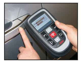
The screen will indicate the signal from the Vehicle and Key Fob, and will show the max output level seen. Use the tool to verify that the Key Fob is working and the Vehicle is sending a signal. Where to place the tool on the vehicle will very slightly, but start around the Drive Side Door handle and just below for outside, and over the center council when testing the Push Button Start.
