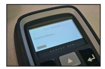
The Bartec 500 and 400PRO is equipped with Wi-Fi connection for easy Tool Updating. Release R53.0 enables this function and allows the operator to connect to their Wi-Fi Network to access the Bartec Tools Server for future updates.
