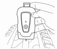
Before completing a Tread Inspection, ensure the pin is pushed out by pressing the manual tread pin down. Ensure the end cap is flat on the tire tread.
