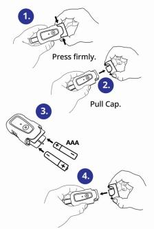
When the tool On/Off light flashes Red the batteries are low and need replacing.
