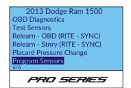
Bartec recommends completing a Relearn following any Wheel and Tire service, including change in air pressure (when the TPMS light will not go off), Tire Rotations, and Replacing TPM sensors.
