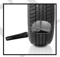
When the OE application is Banded (Ford) the tool will need to be positioned 180 degrees opposite the valve stem, when the OE banded sensor is fitted. (Banded sensors can be replaced with valve mounted Aftermarket Sensors)
