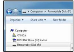
Copy/paste or drag and drop the saved update file (\*.mfu) into the Removable Disk window. Once file copying is completed, disconnect the USB cable from the tool.
