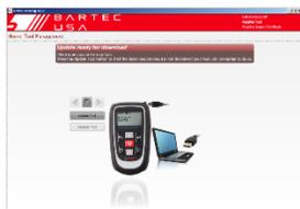
To continue with the update, your tool must be in “update mode” – follow the on screen (PC) prompts to place your tool in update mode. With the tool connected and updating, the user will be guided through the updating process.
