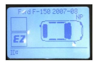
If using EZ-sensor<sup>TM</sup>, and you get NP as shown here, you have programmed the sensor as a LOW PRESSURE range, and the sensor has been pressurized over 50 psi.
