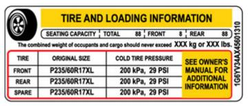
If the vehicle placard calls for any pressures to be higher than 50PSI, you will need to use the HP (High Pressure) TPMS Sensor.
